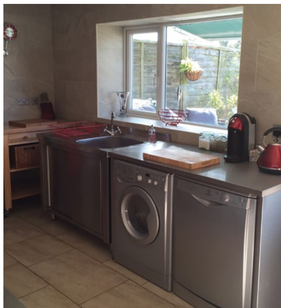
Figure 4 Free-standing stainless steel kitchen with free-standing appliances, which can therefore be moved to safety. The walls are tiled from floor to ceiling, using water-resistant cement and grout; internal door re-hung with hinges allowing it to be lifted off and moved upstairs.
